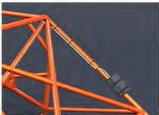
Connecting Cable – routed on inside of roll cage in order to avoid damage in event of car rolling etc.
